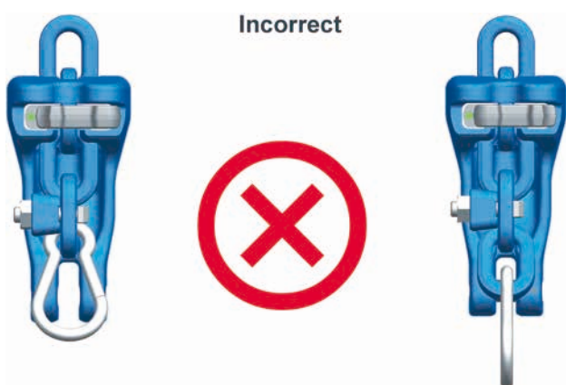
Figure 11 – Incorrect assembly of the stopper set
